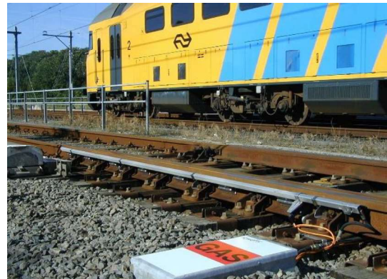
Figuur 2.4 Gas lintelement (Wikipedia, 2010a)
